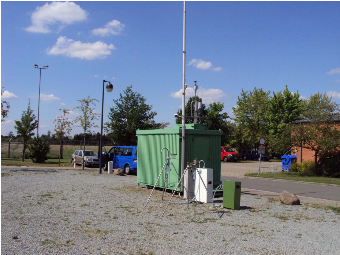
Figure S1: High volume sampler deployed at reference site in region Wendland.
