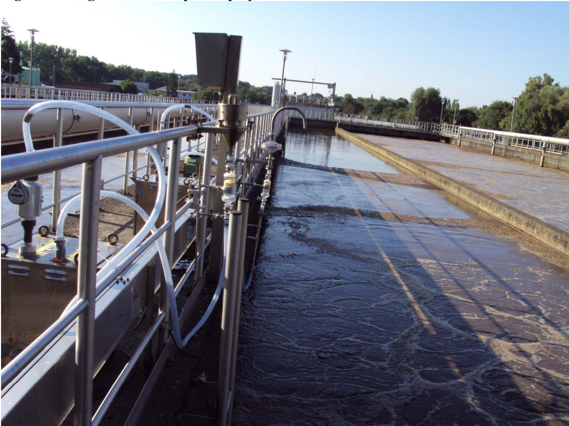
Figure S4: High volume sampler deployed at waste water treatment plant WB.
