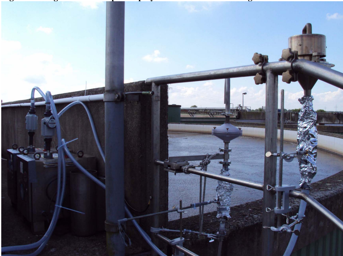
Figure S2: High volume sampler deployed at waste water treatment plant WA.
