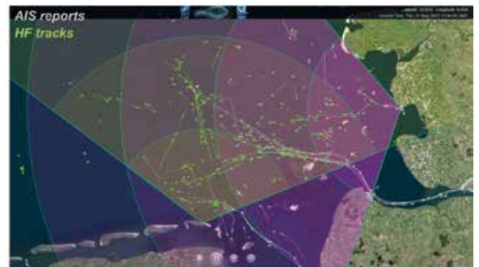
Example of resulting ship tracks after tracking and fusion of 30 minutes of HF-radar data collected on 1. August 2013. The data provided through this source complements official sources based on AIS reports.
