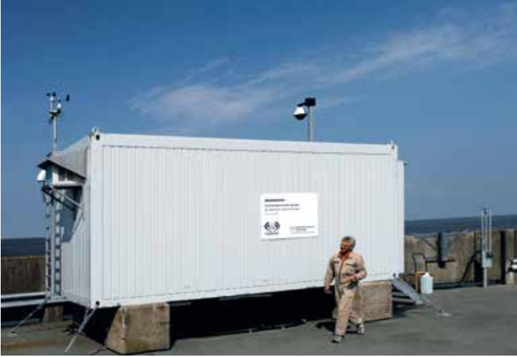
The stationary FerryBox located in a container in Cuxhaven, Germany at the mouth of the River Elbe. (Photos: HZG)
