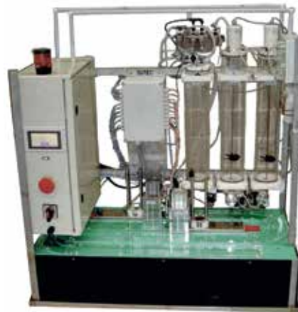
Automated filtration unit for processing filtered algae prior to detection by the biosensor (Photo: ISITEC)
