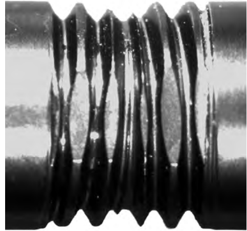
(b) Empirically designed threaded bobbin tool pin (as manufactured)
