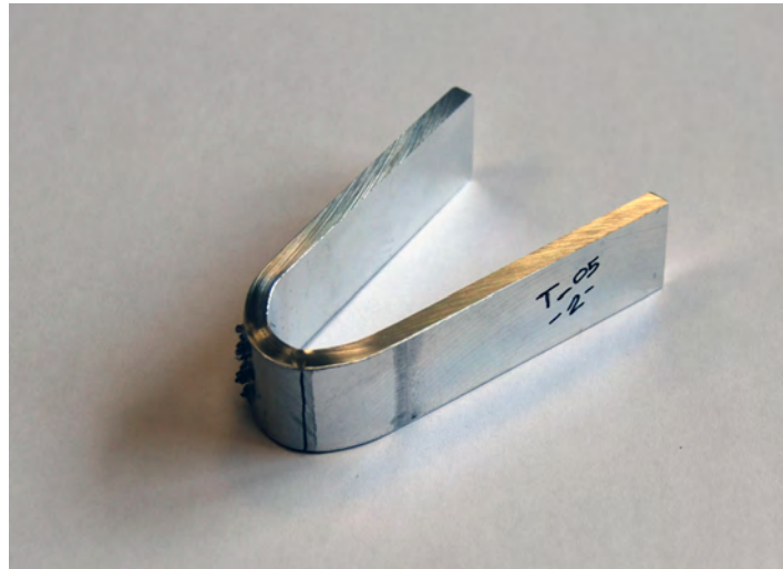
Figure 7.3: Extended bending specimen (T_05)
