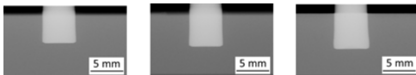
Figure B.1. X-ray scans of FricRiveted metallic-insert joints made of PEEK and grade 3 titanium and joined using configuration 1 (see Table 5.1)
