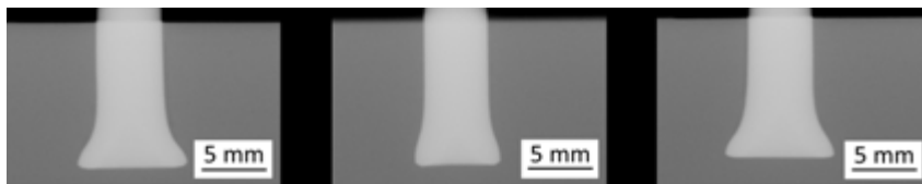
Figure B.16. X-ray scans of FricRiveted metallic-insert joints made of PEEK and grade 3 titanium and joined using configuration 16 (see Table 5.1)
