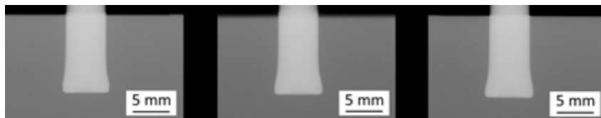
Figure B.11. X-ray scans of FricRiveted metallic-insert joints made of PEEK and grade 3 titanium and joined using configuration 11 (see Table 5.1)
