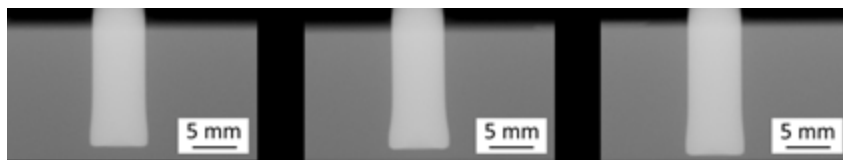
Figure B.10. X-ray scans of FricRiveted metallic-insert joints made of PEEK and grade 3 titanium and joined using configuration 10 (see Table 5.1)
