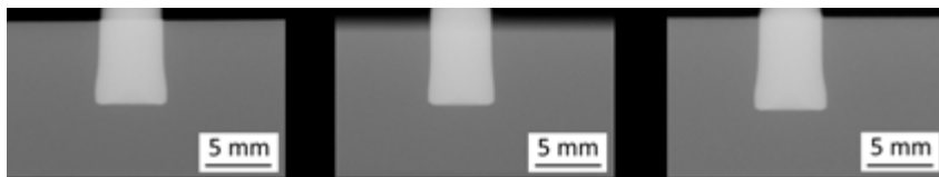
Figure B.3. X-ray scans of FricRiveted metallic-insert joints made of PEEK and grade 3 titanium and joined using configuration 3 (see Table 5.1)
