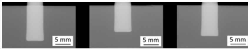
Figure B.9. X-ray scans of FricRiveted metallic-insert joints made of PEEK and grade 3 titanium and joined using configuration 9 (see Table 5.1)
