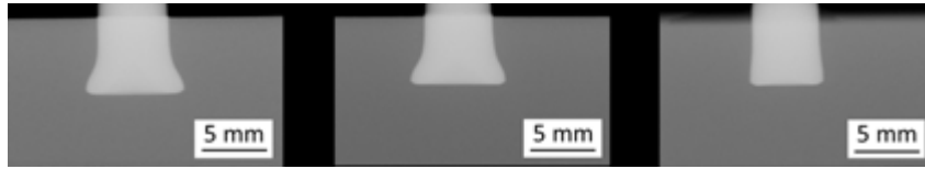
Figure B.7. X-ray scans of FricRiveted metallic-insert joints made of PEEK and grade 3 titanium and joined using configuration 7 (see Table 5.1)
