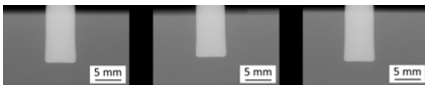
Figure B.6. X-ray scans of FricRiveted metallic-insert joints made of PEEK and grade 3 titanium and joined using configuration 6 (see Table 5.1)
