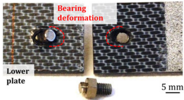
Figure 7.13. Example of a friction-riveted single-lap shear joint ( w/d = 6 ) failing by mixed bearing/rivet failure mode
