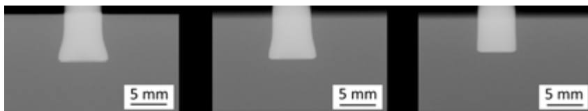
Figure B.5. X-ray scans of FricRiveted metallic-insert joints made of PEEK and grade 3 titanium and joined using configuration 5 (see Table 5.1)
