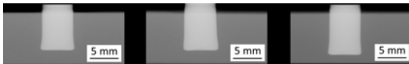
Figure B.14. X-ray scans of FricRiveted metallic-insert joints made of PEEK and grade 3 titanium and joined using configuration 14 (see Table 5.1)
