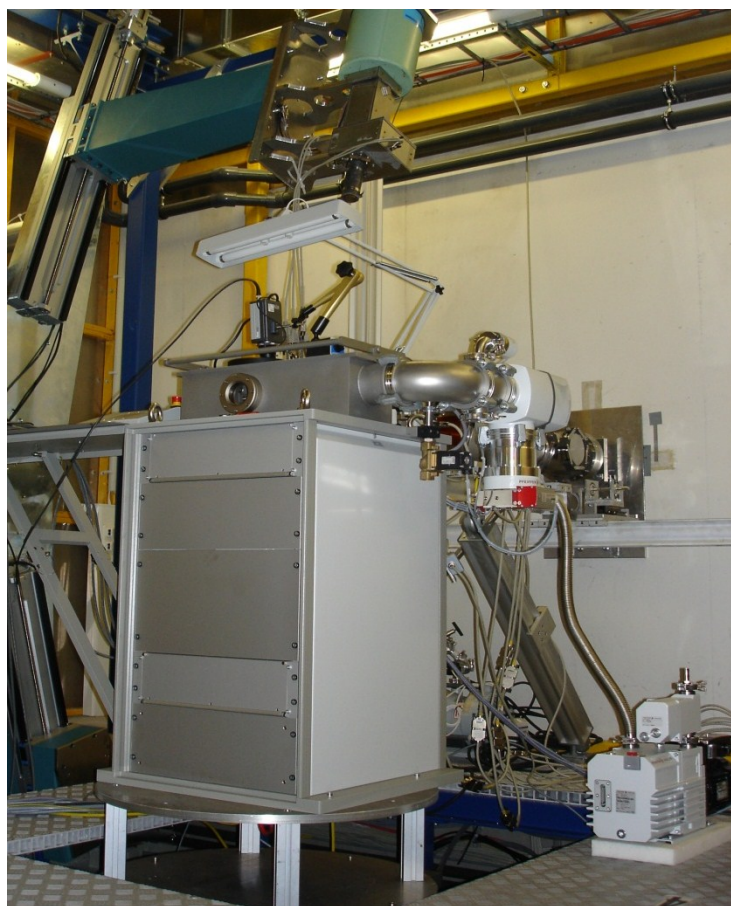
Figure 2: Deformation dilatometer mounted at the beamline
