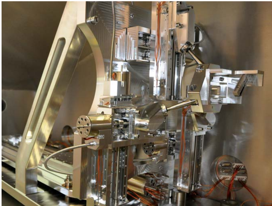
Figure 5.10: View of the in-vacuum lens positioning mechanics, as mounted in the vacuum chamber. The base plate is visible at the bottom inside the chamber. The mechanics are mounted on this plate to prevent bending due to the bending of the chamber walls if evacuated. To the right, the kinematics for lens positioning are visible; to the left in the background, the long translation in beam direction for slits or diagnostics. The retractable photo diodes are not visible, they are mounted directly on the chamber walls next to the entrance and exit pipes. To the very right, the adapter for the lens and two lenses are mounted on the kinematics.
