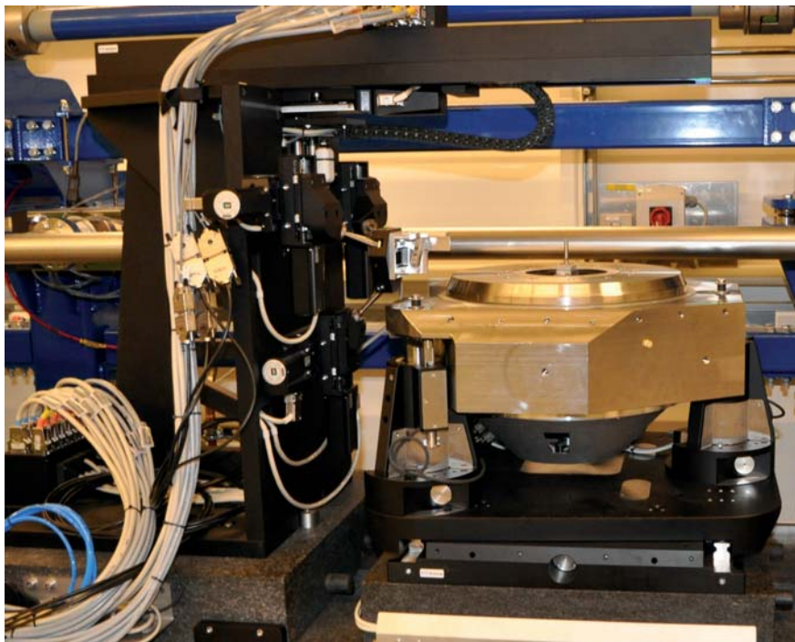
Figure 5.15: Photograph of the optics station, mounted in the X-ray microscopy orientation. The optics station is shown to the left and top of the image. The SpaceFab kinematics is mounted on the central support and the X-ray lenses are mounted on the flyer (center of the image). The cross bar is visible at the top and is used for installing the apertures and photo diodes (hidden from view).
