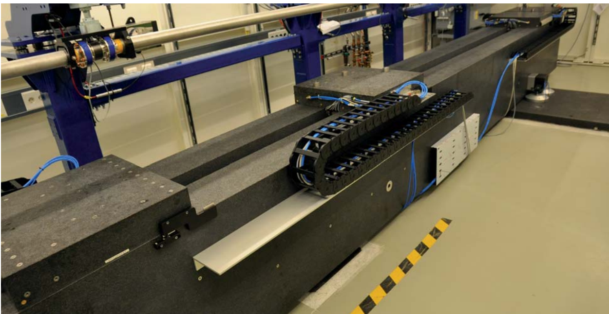
Figure 4.3: The granite substructure for the experiment. A 6.8 m long granite slab acts as optical bench for the experimental installations. On the right side in the background is the granite ground plate for a horizontal translation of the complete substructure on air pads. This is necessary for removing the experiment from the beam path to install the vacuum pipe.
