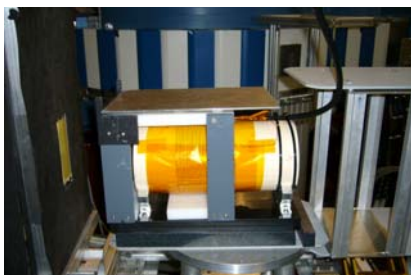
Fig. 0.3: Spin Flipper set up installed for a first test at the instrument MIRA.
