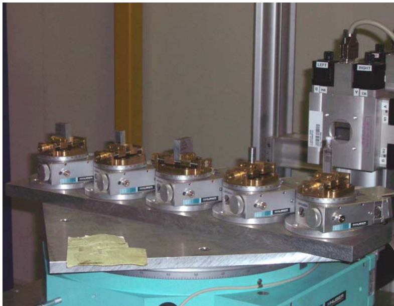
Fig. 1: Set of investigated Al7020 samples mounted on the new sample changer at Harwi-II
