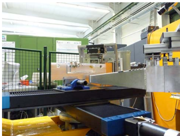
Figure 1: Three ESET samples mounted in the diffractometer.
