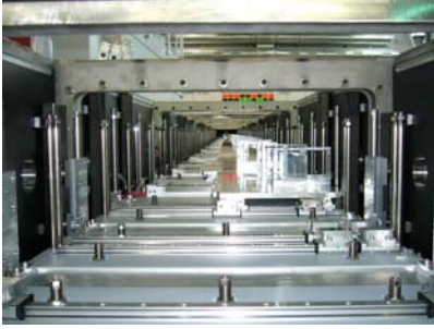
Fig. 0.4: The inner life of the collimation system with movable tables to position various components in the neutron beam.
